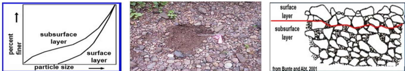
Figure 1: Streambed material is made up of surface and subsurface layers. The surface layer is typically coarser than the subsurface layer because of the scour of fines between the larger particles. The subsurface layer is finer than the surface layer because fines are present in the voids between the larger particles.
