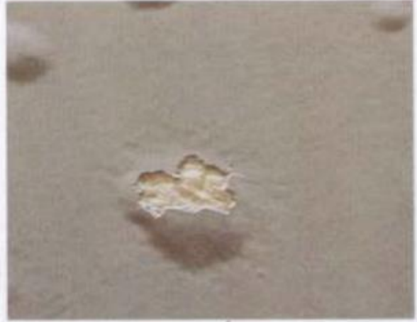
4. Blisters — caused by catalyst drop
