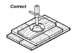
To avoid crushing under load "crib" blocking should be spaced no more than 1/4" for drainage.
