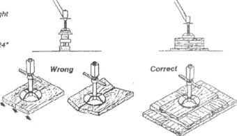
To avoid crushing under load "crib" blocking should be spaced no more than 1/4" for drainage.
